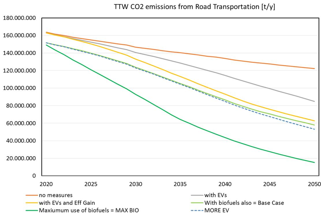
Figure 50: TTW CO<sub>2</sub> emissions evolution by different measures in road transport for Germany in the MAX BIO scenario.
