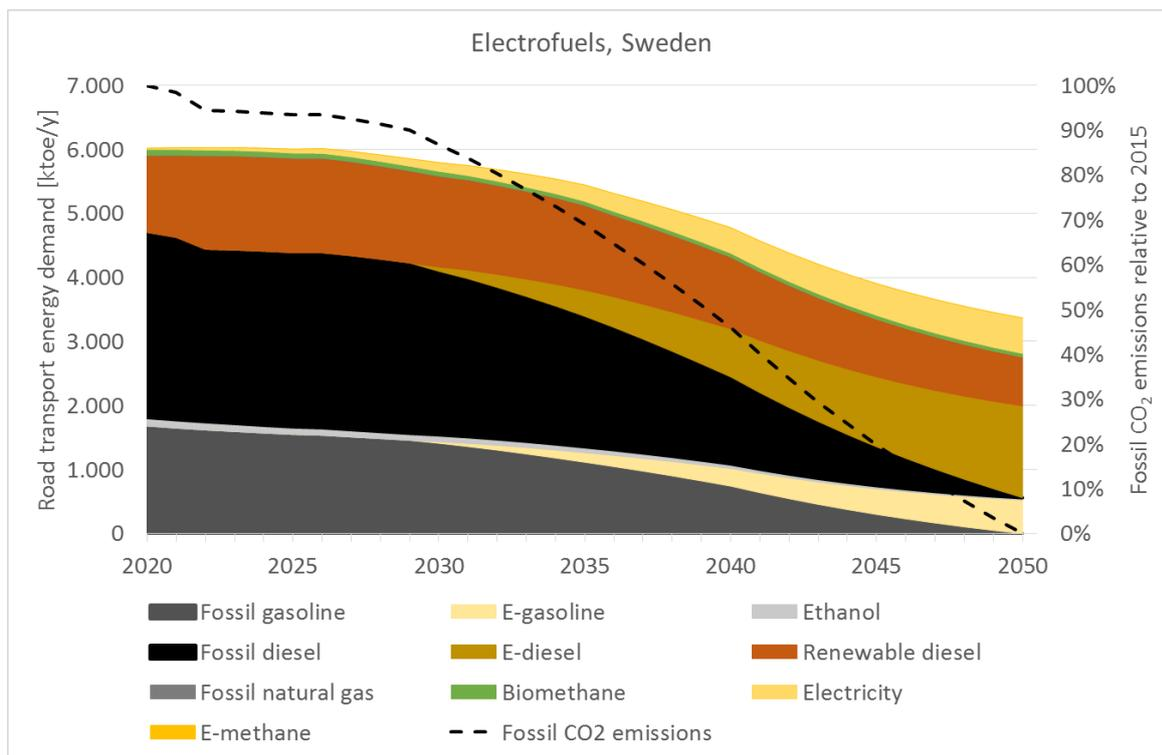
Figure 56. Energy use in road transport by energy carrier for Sweden in the E-FUELS scenario.
