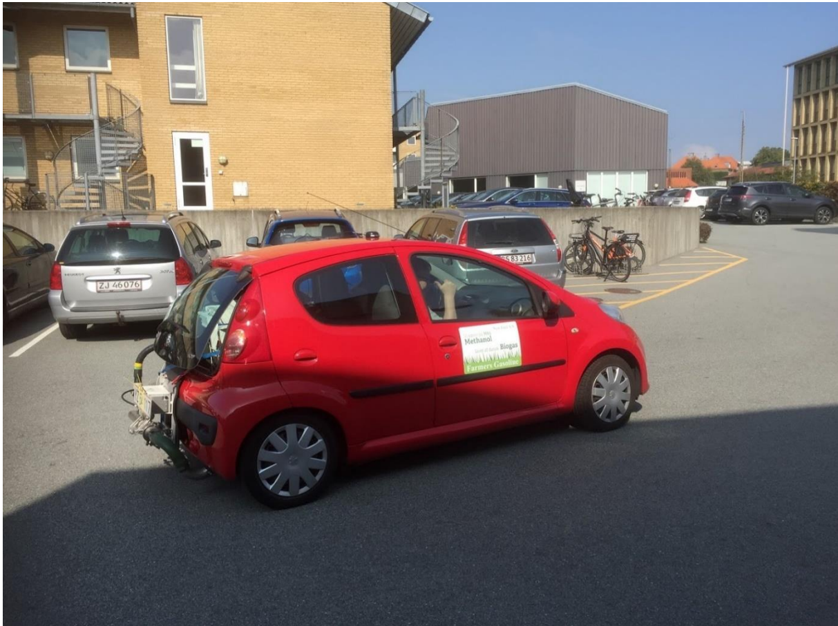
Figure 1 Test vehicle equipped with measurement system
