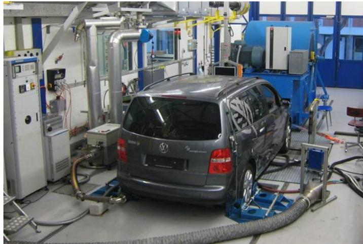
Fig. CS3.1 Project vehicle on chassis dynamometer
