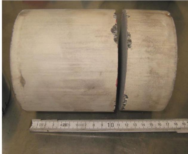
Fig. CS3.2 Shortened catalytic converter - only the left part (2/3 of the length) was used.
