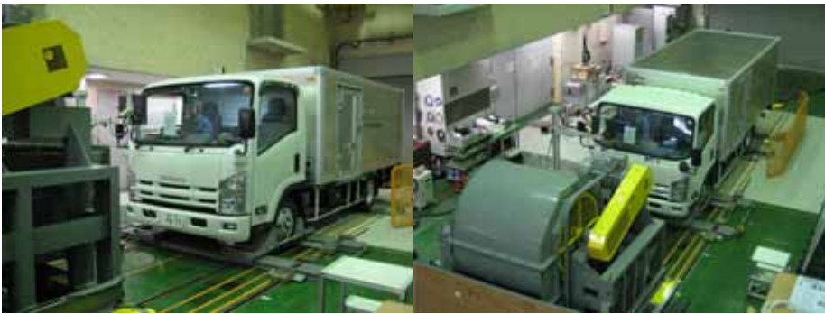
Figure 4-2 Test vehicle set on the chassis dynamometer
