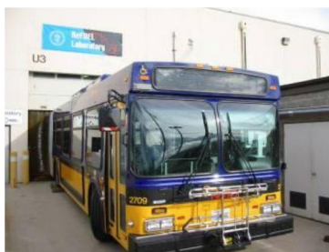
Figure 8: GM-Allison hybrid transit bus at the NREL ReFUEL Chassis Dynamometer Test Facility
