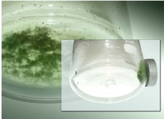
Figure 12: Biomagnetic separation of algae from water using finely ground iron oxide, at the bottom of a flask (Image Source: Siemens AG).
