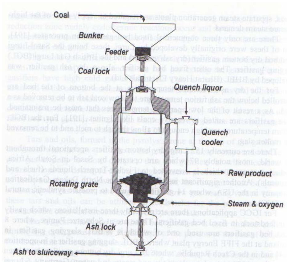
Figure 1 Sasol-Lurgi fixed bed dry bottom gasifier [7]
