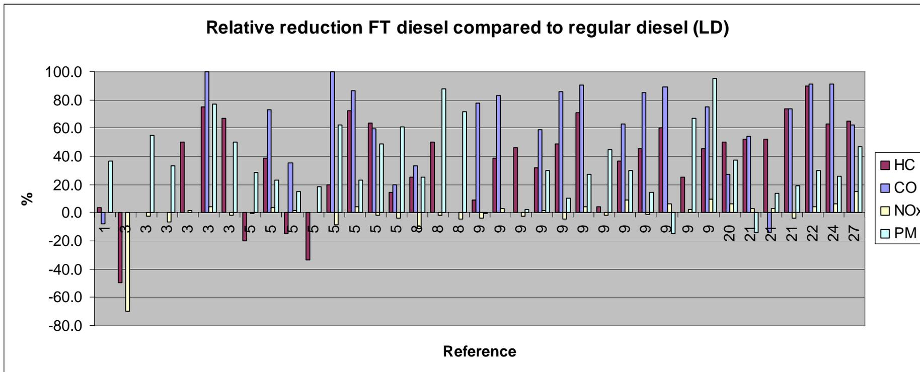
It is seen from the figure that HC, CO and PM emission is significantly reduced using synthetic FT diesel. NOx emission is in many cases not reduced at all. Negative reduction means that FT diesel causes more emission than with conventional diesel.
