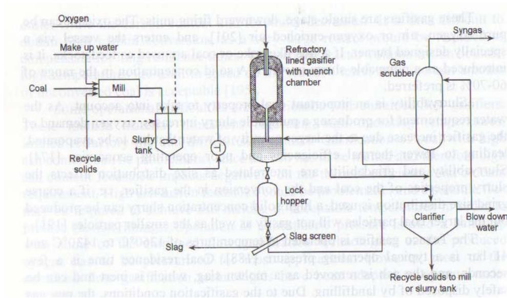
Figure 3 Texaco gasifier with quenching [9]
