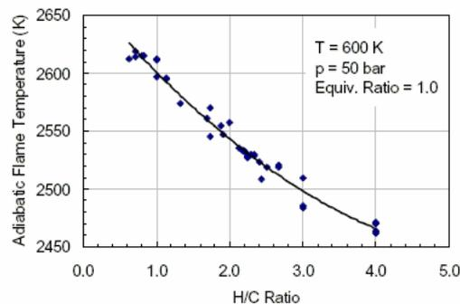
Calculated adiabatic flame temperature as a function of atomic C/H ratio for a variety of hydrocarbon fuels
