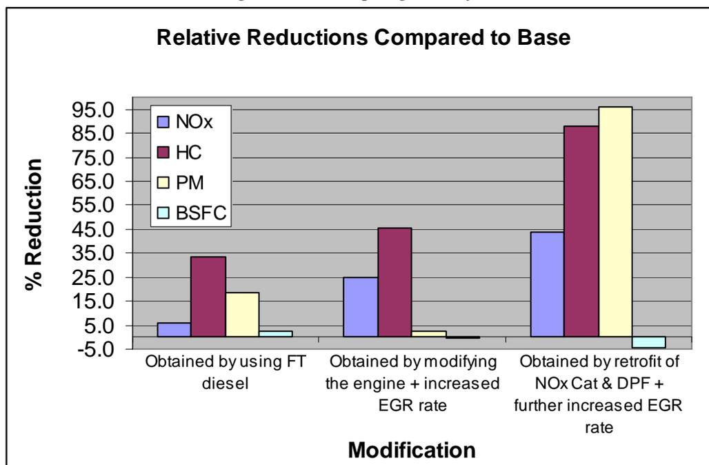
A presentation [28] of emission data comparing emissions from a 2002 Cummins ISM heavy duty engine with EGR fueled by a high quality baseline conventional diesel and a FT diesel. The conventional diesel had 8.1% aromatics and The FT diesel had less than 0.1%. Both were very low on sulfur. The reductions caused by changing fuel were 5.5, 33.4 and 18.7% for NOx, THC and PM respectively. A modification of the combustion bowl of the piston was
