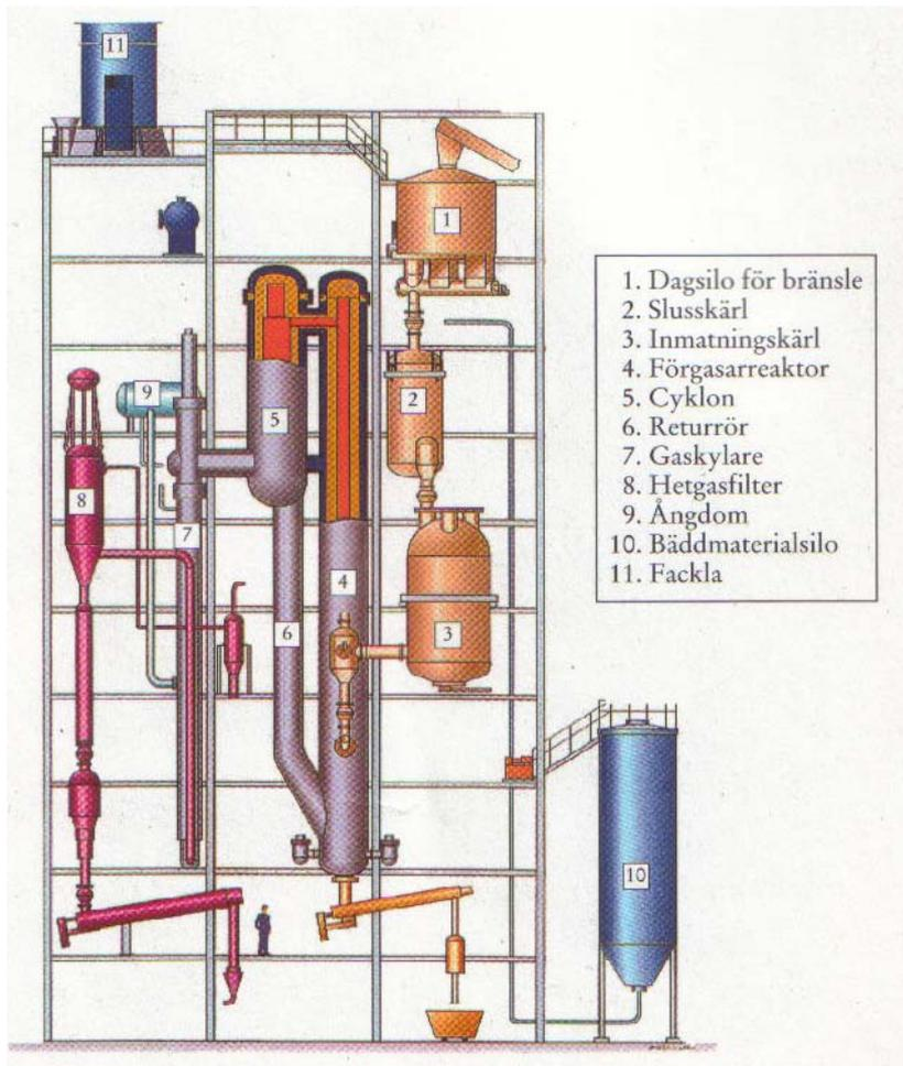
Picture 8 Gasification plant, Värnamo Plant, Sweden [13]
