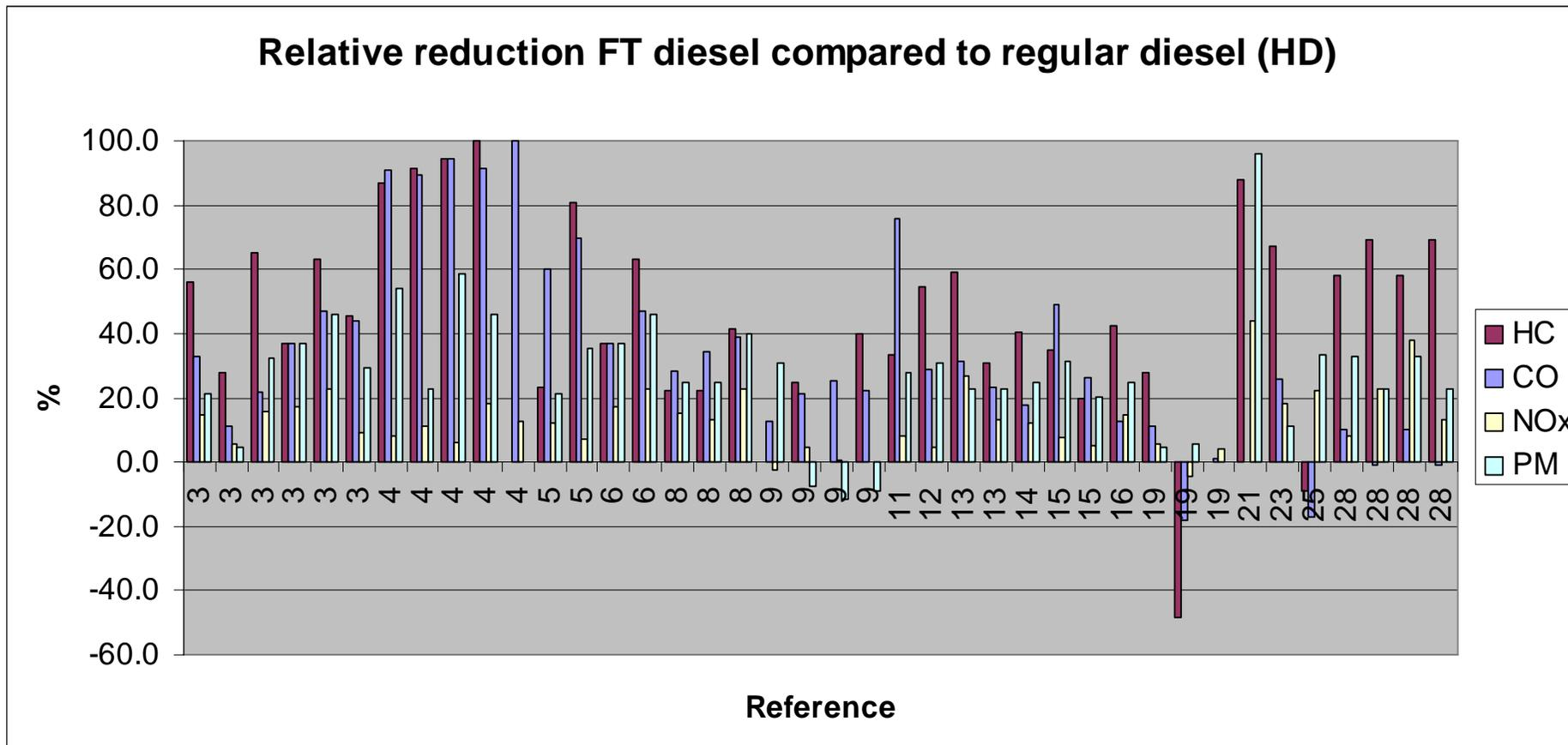
The figure shows that CO and HC emission is reduced significantly with the use of FT diesel, while NOx and PM emission is reduced to a lesser degree. It also shows that emissions are reduced in almost all of the investigated tests with only a few exceptions.
