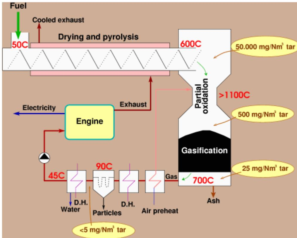
Figure 4 Two-stage gasifier
