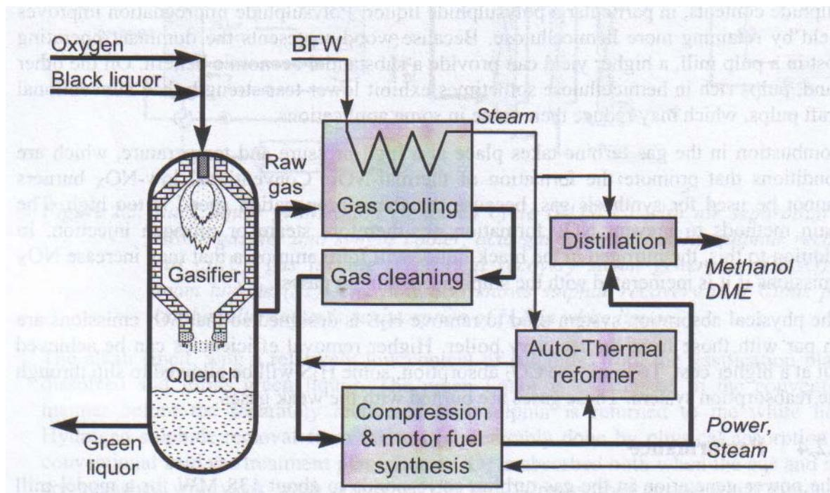
Figure 11 Black liquor gasification with motor fuel production (BLGMF)
