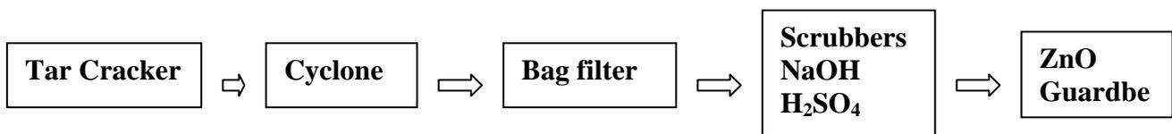
Wet gas cleaning can be said to be the conventional way of cleaning synthesis gas for use in gas turbines.
