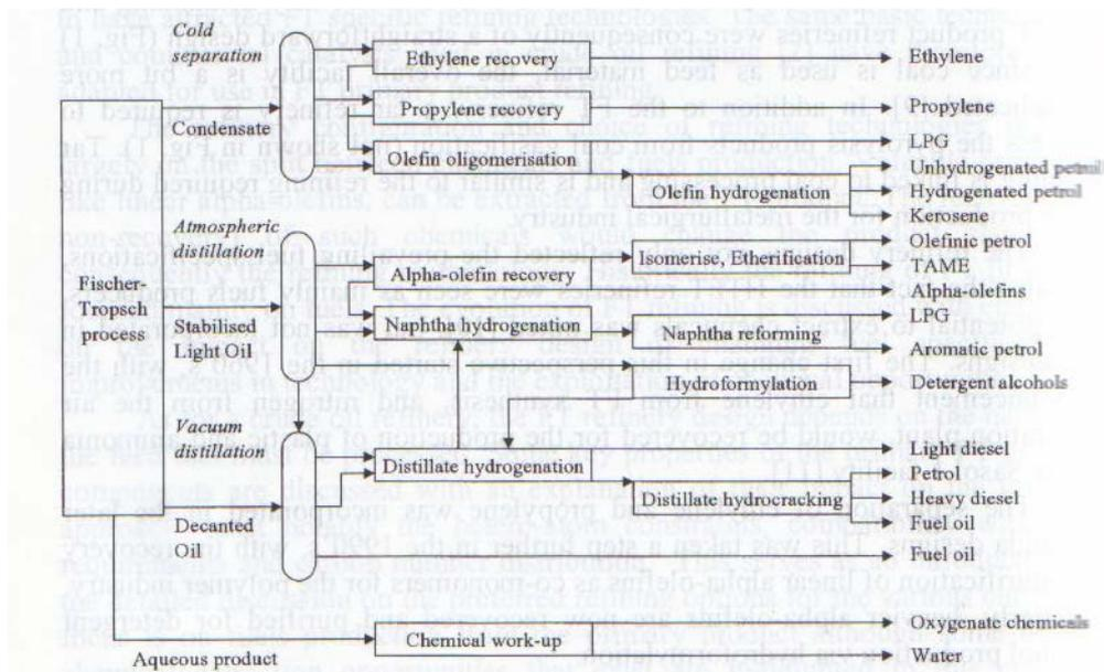
Figure 14 The 2004 design of the HTFT refinery used at Sasol's plant Secunda, South Africa [6].
