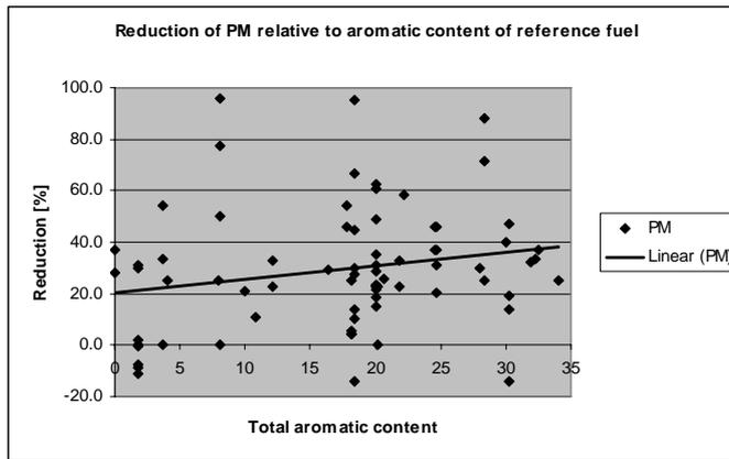
Figures 28 – 31 Relative reductions of pollutants NO<sub>x</sub>, CO, HC and PM relative a normalized aromatic and sulfuric content.
