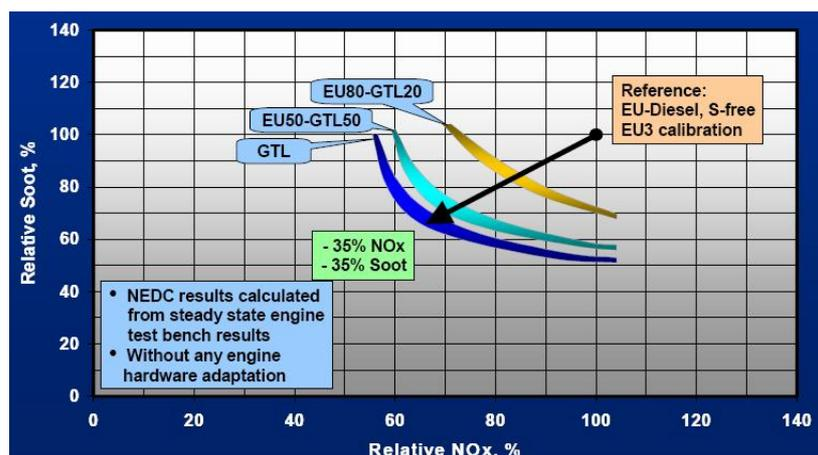
Soot and NO<sub>x</sub> emission reductions (compared to the reference) of 35, 30 and 15% for neat, 50/50 and 80/20 fuels respectively were obtained by recalibration and optimization of the ECU. See figure 29. It was concluded that blends of EU and GTL diesel might show reductions significantly larger than the blending ratio. 40% of the emissions benefit of GTL may be obtained in a 20% GTL blend and up to 85% may be obtained in a 50% blend.
